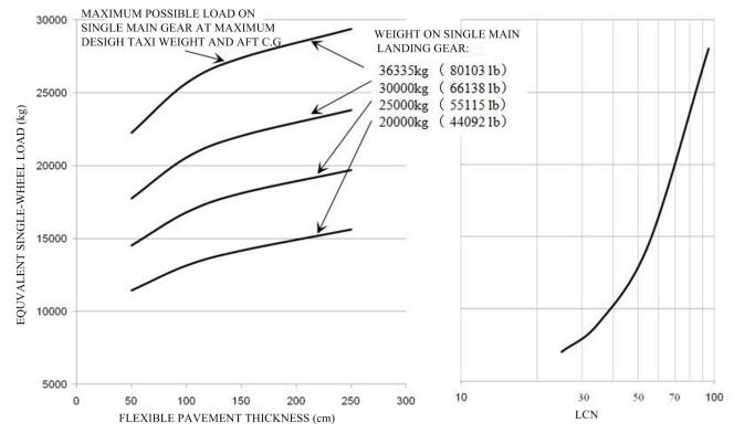
Note: Main Landing Gear Tires are 46\*17R20/30PR, pressure holds on 187psi. Equivalent single-wheel loads are derived from ICOA AERODROME MANUAL, PART 2 PAR.4.1.3.
