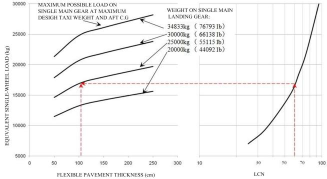
Note: Main Landing Gear Tires are 46\*17R20/30PR, pressure holds on 187psi. Equivalent single-wheel loads are derived from ICOA AERODROME MANUAL, PART 2 PAR.4.1.3.
