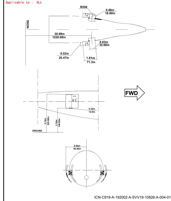
Figure 5 After Service Door Clearances (Sheet 1 of 1)
